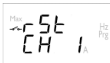
Channel tripped off
