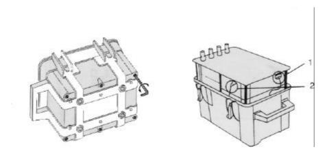
Lift away the chassis without forgetting to disconnect the linking cables 1 and 2 connecting the power
