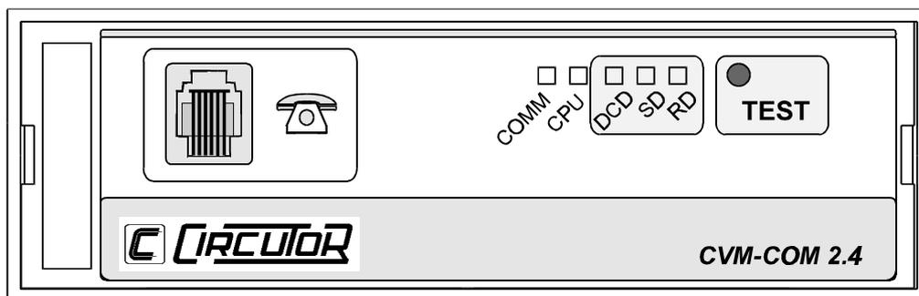
a.- "**COMM**" LED: This led blinks when the peripheral is receiving data from the CVM ("Network") or from the PC. When no communication exists the led is lit off.
